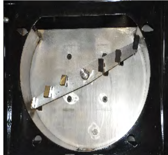
No Dead Space Mixing Chamber With Welded Single Piece Scroll
